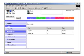
**Tray:** The names of optional trays that are installed are
